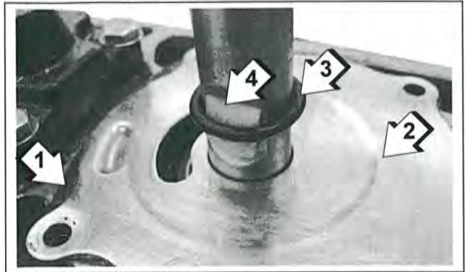
1. Impeller plate gasket 2. Impeller plate 3. O-ring 4. Impeller key 006871
